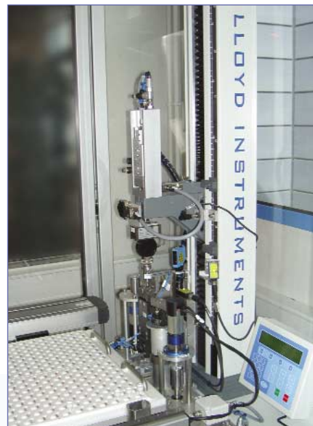
Automated sample handling system
